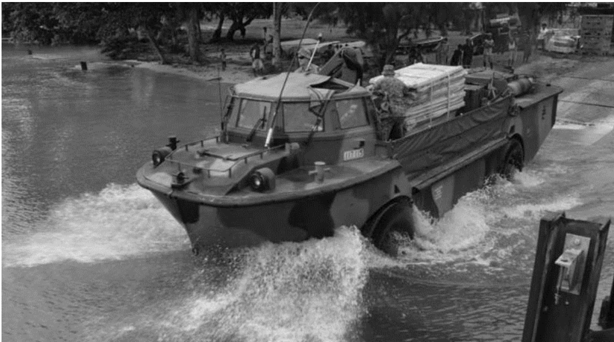
Papua New Guinean children watch a LARC-V retrieve Australian Defence Force equipment from Manus Island. Note the cargo carrying capability of the vehicle. Photo: Royal Australian Navy (RAN)
