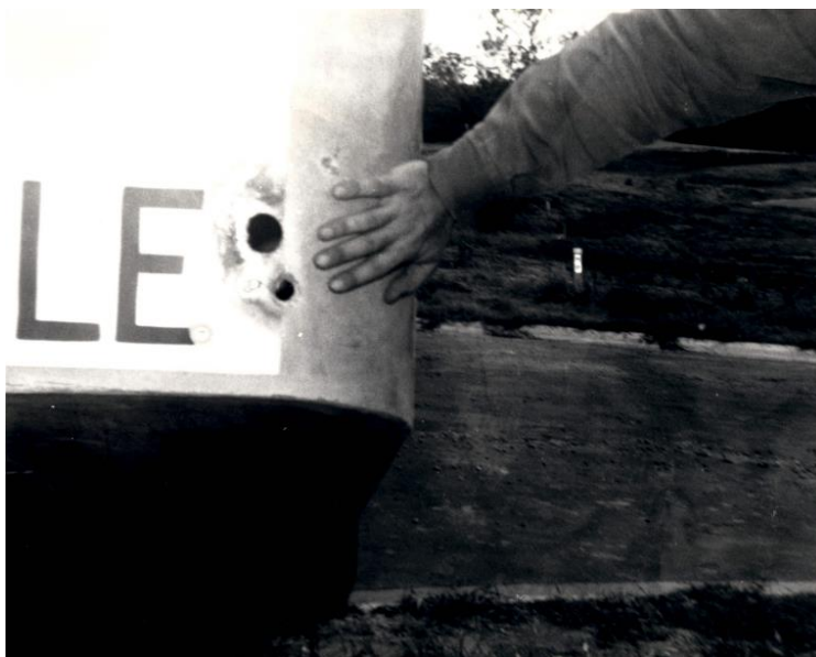
The electricity passed through the aluminium hull of the LARC and punched two holes in the rear of the vehicle. Photo: Army Court of Inquiry. NAA ID 32538534
