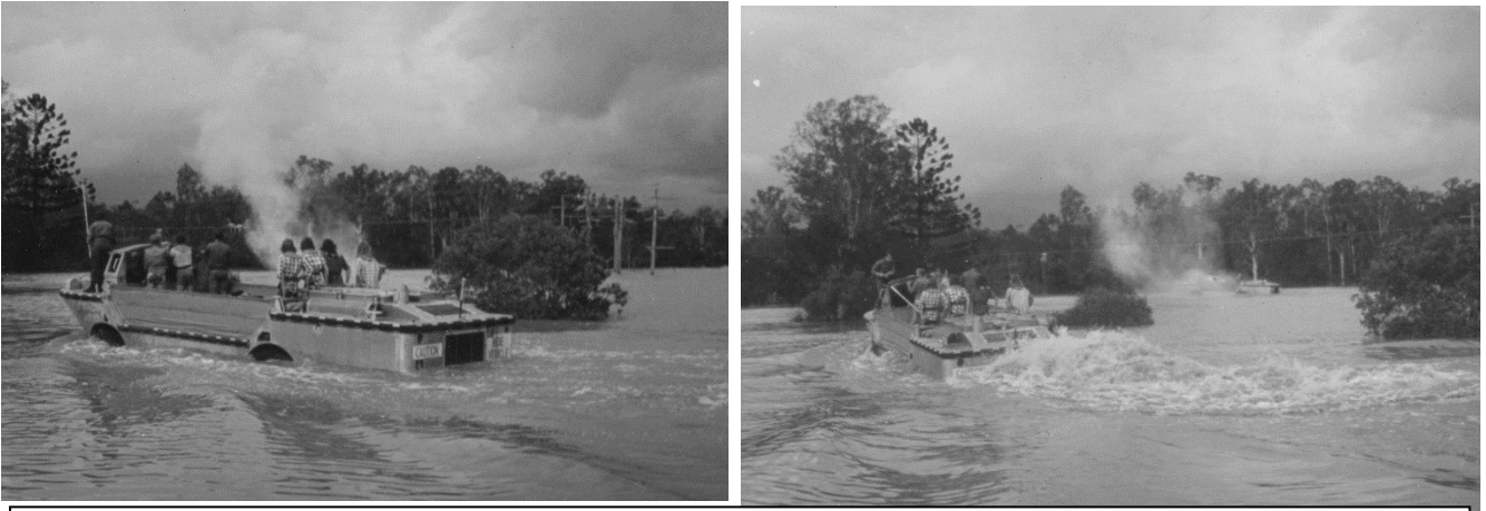
Photographs taken immediately after LARC 05 had contacted the power supply. Smoke is being emitted from the vehicle. LARC 09, which had been following the stricken vehicle, is in the foreground. Photos: Roger Todd
